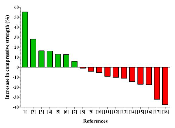
Figure 3 - Increase and decrease (percentage) in compressive strength of cementitious materials made with bamboo ashes in comparison to reference samples
